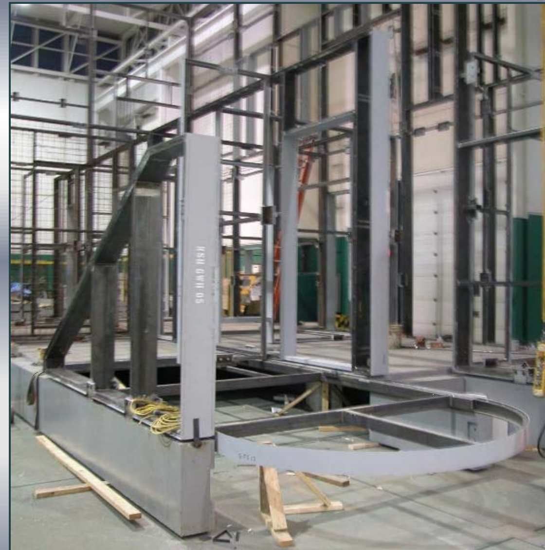
A PERSPECTIVE VIEW OF THE CURVED LANDING IN THE STAIRCASE AT ONE END.
